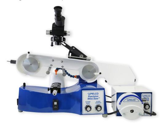
The PELCO<sup>®</sup> Precision Wire Saw™ is capable of cutting a variety of materials while minimizing damage from the cutting process using a gentle lapping action. This gentle action combined with high precision and low kerf damage makes the Diamond Wire Saw ideal for slicing samples
