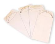
The PELCO® Precision Wire Saw™ uses wire loop blades. Either Diamond-embedded Stainless Steel wire blades or plain Stainless Steel wire blades may be used, depending on whether an abrasive slurry is used for cutting. Blade diameters of 0.010 and 0.015" are available. The wire blades can be easily changed and appropriately tensioned within a few moments.
