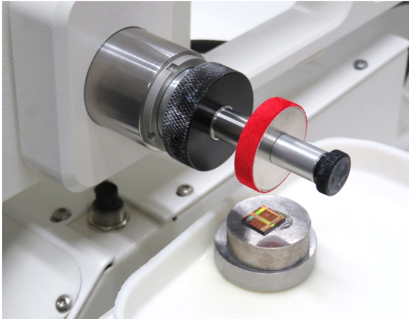
Figure 7: Platen and Tool on the PELCO® Dimpler™
