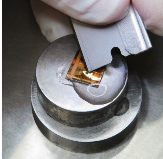
Figure 3: Removing the Passivation with a Razor Blade
