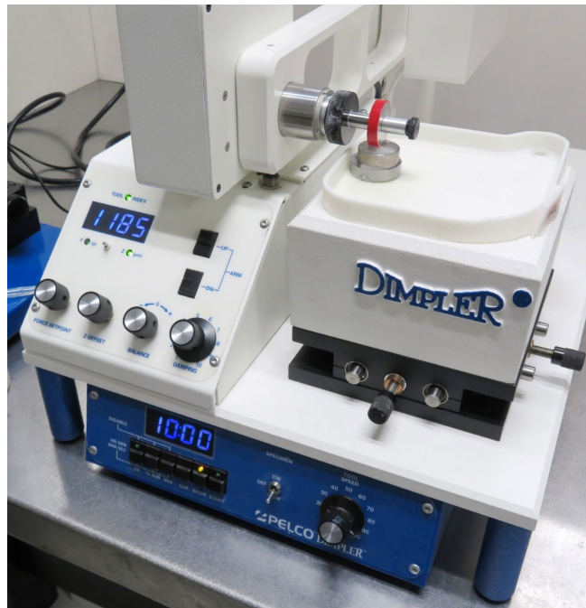
Figure 9: Dimpling the Sample
