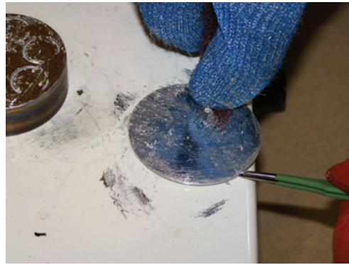
Fig. 6 Transfer indium to new target
