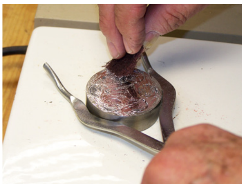
Fig. 5 Smooth indium with Scotchbrite™
