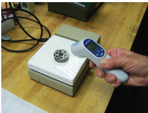
Fig. 1 Heat to 170°C
