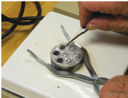
Fig. 4 Remove residue target material
