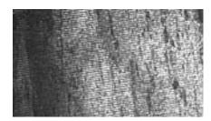
Beef liver catalase crystals have lattice spacings of 8.75nm and 6.85nm. These are easily visible, and can be used to calibrate the upper end of the magnification range of a microscope.
