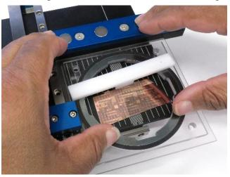
Figure 9: Sample in Wafer Holder Placed onto the PELCO® FlipScribe®
