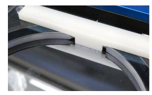
Figure 4: Lip in Clamping Bar Seated onto Wafer
