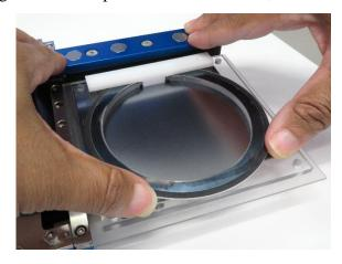
Figure 6: Scribing a Wafer using Wafer Holder
