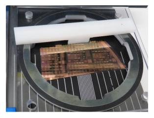
Figure 8: Clamping Bar Positioned to Hold Sample in Place
