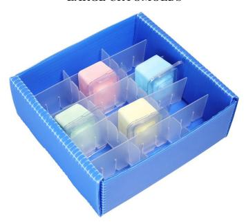
To configure the True North® Freezer Box for large cryomolds, remove all vertical dividers from the insert except the 3<sup>rd</sup> and 6<sup>th</sup> one. Then, remove every other horizontal divider.
