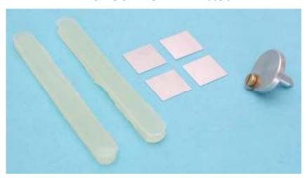
A thermoplastic adhesive for mounting powder specimens and small particles for scanning electron microscopy
